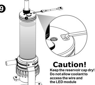
After adding the recommended coolant, remember to fill the reservoir to only 80% and leave the fill port cap off. This will help stabilize your internal loop pressure
