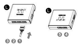
Connect the reservoir cable onto the controller.
