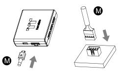
Connect the controller cable onto the mainboard (USB 2.0 9 pin) and controller.
