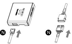
Connect the power cable to the 4pin Molex
